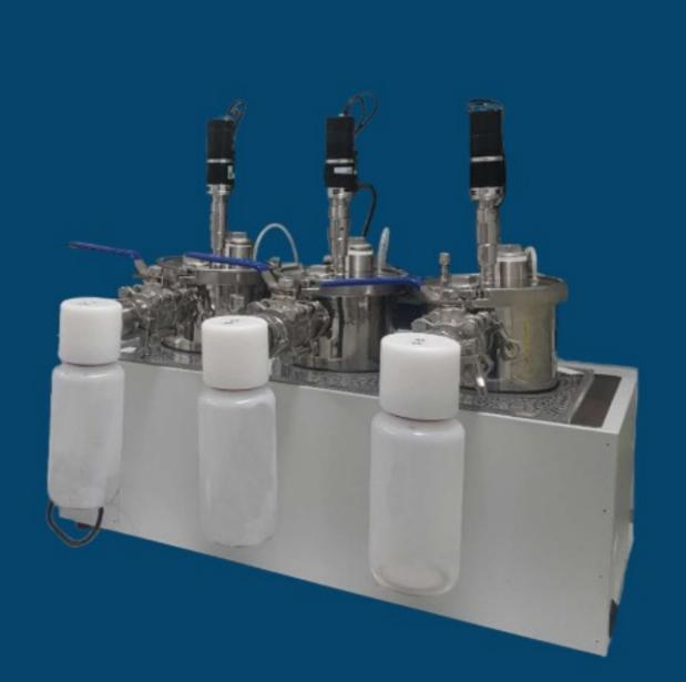
The Pegasus is our second batch-fed model, featuring 5/10L reactors. With up to 18% dry solid substrate having been used before, these larger capacity digesters enable the use of more fibrous and solid content that would be unsuitable for automatic feeding - as well being easier to operate with (less spillage when feeding).
