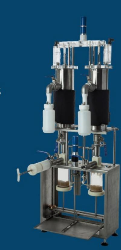
The Ray is an ideal auto-fed machine when a large amount of reactors is not necessary. Compatible with up to 20L reactors, large volumes of feedstock can be tested, with potential for later upgrade to become a multi-stage system. The Ray-i is the upgraded model which includes an automatic-feeder with each reactor, so feeding can be performed individually at controlled rates.
