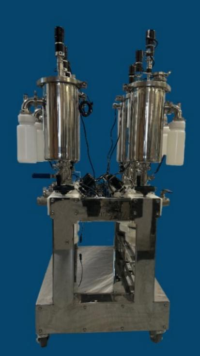
From our automatic range, the lobster model is equipped with six, 5 litre reactors (smaller options available). With an adjustable rate between 0 and 999 feeds a day, and the capability to use mixed fluid feedstocks from AD plants directly, the lobster can closely simulate the feed of an industrial AD plant.
