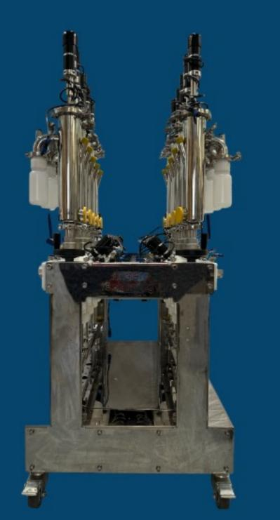
The Caterpillar offers massive research capabilities partnered with ease of use. The 10 automatically fed reactors, operating with individual temperature control, provide the capacity for multiple experiments - a valuable tool if there are various ongoing projects, or to compare differences in a particular substrate's biogas productions.
