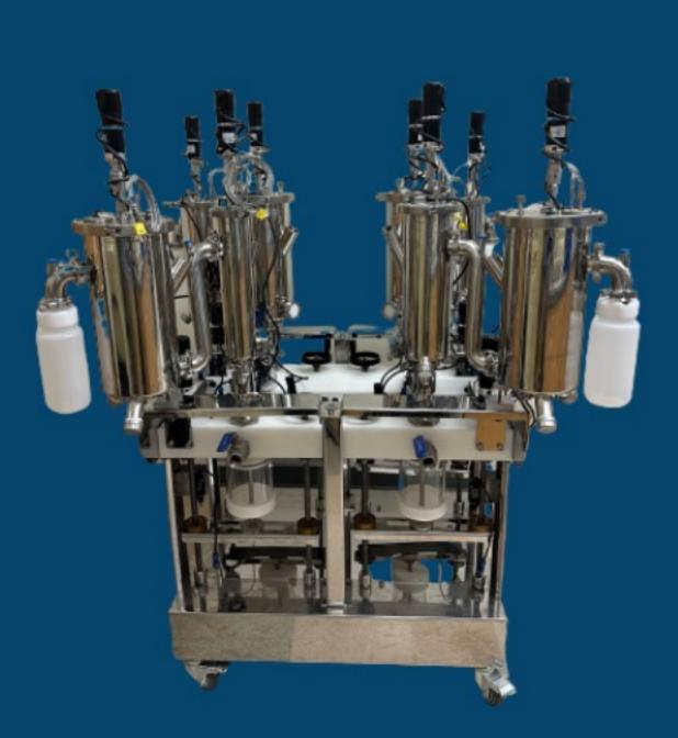
Boasting many possible configurations, the Black Swan is our most comprehensive multi-stage model. With four 1st stage and four 2nd stage reactors (+optional additional stages), and 4 auto-feeders, the Black Swan allows you to compartmentalise the AD process by configuring each stage through temperature control and HRT.
