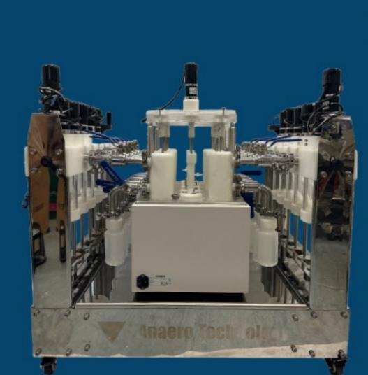
Also available as an upgrade to current BMP's, the Medusa is a hybrid system, with 10 automatically fed and 5 batch fed reactors. Suited to fibre-free or slurry feedstocks and covering both feeding regimes, the Medusa can perform versatile research particularly into microbial kinetics due to its many possible feedings configurations.
