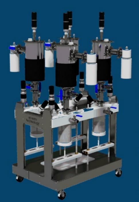
The Lobster-i model features 5 litre reactors (smaller options available), but with more flexibility for the feeding rate since each of the 4 reactors is equipped with its own feeder. This means 4 independent tests can be run simultaneously from the same machine. The Lobster and Lobster-i can both later be converted to multi-stage systems.
